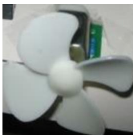
Figure 3 DC Motor with Fan blades.
